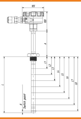
L= up to 6 000 mm (for rod sensor) L= up to 20 000 mm (for flexible sensor)
